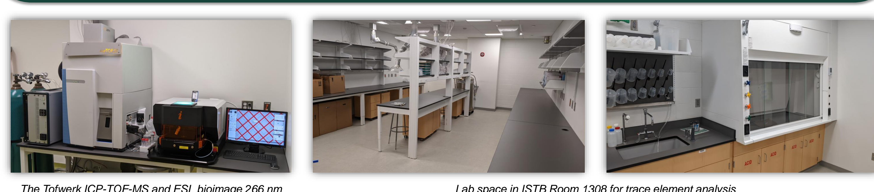
The ToFwerk ICP-TOF-MS and ESL bioimage 266 nm laser ablation system setup in ISTB Room 1307. Lab space in ISTB Room 1308 for trace element analysis.
